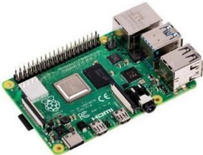
Fig 30. Raspberry PI model 4 selected to process the multimodal panel information
